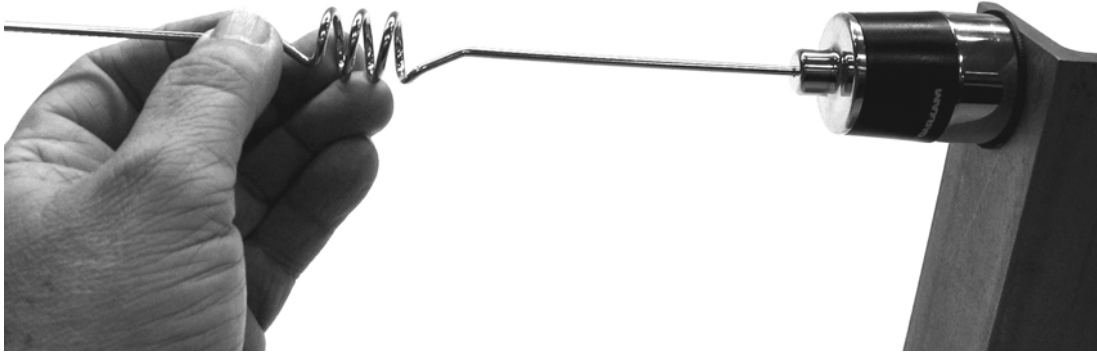
Figure 2 Whip Antenna Inserted into Collar
