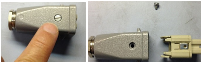
Figure 10 Remove Screw and Plug Insert
