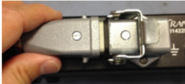
Figure 23 Remove Plug from Receptacle
