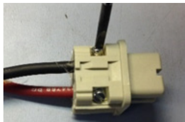
Figure 15 Thread Wires Through Assembly
