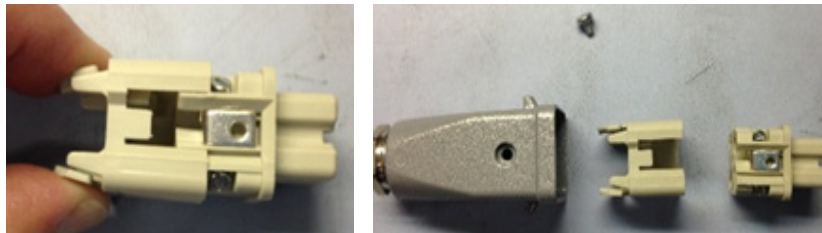
Figure 11 Remove Wire Harness from Insert Clip
