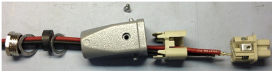
Figure 14 Thread Wires Through Assembly
