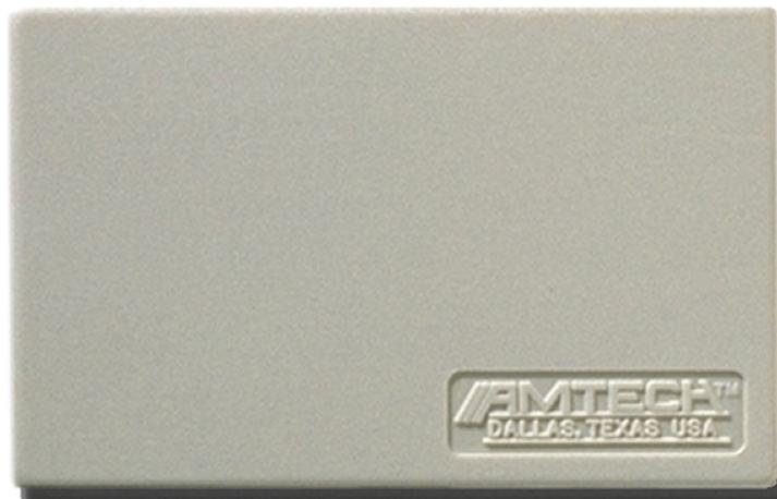
The AT5400 TollTag is a full frame, beam-powered radio frequency (RF) tag used in automatic vehicle identification applications with TransCore's Amtech-brand and TransCore Encompass multiprotocol reader systems. This tag is designed for interior mounting on a nonmetallized windshield.
