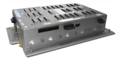
TransCore's Encompass<sup>®</sup> 5 Multiprotocol Reader is an integrated non-toll, multi-protocol 915 MHz radio frequency identification (RFID) reader system that includes an RF transceiver board and processor in a single assembly. The Multiprotocol Reader is ideal for non-toll, multi-lane installations with a requirement to read two tag protocols or to provide a migration path from an existing tag protocol.
