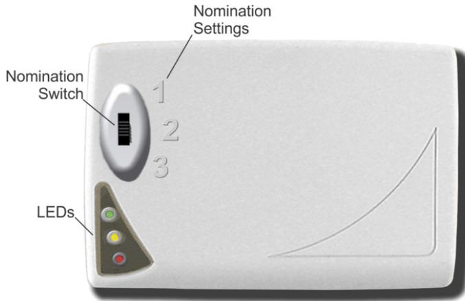
The IT2231 Multi-Purpose Switchable Tag uses a three-position switch to trigger a change from one nomination mode to another.
