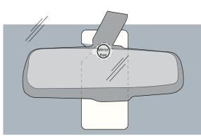
Hook the hang tag over the rear view mirror post. Ensure that no stickers or other objects obscure the hang tag. The hang tag should not be used if other RFID transponders are present on the windshield.
