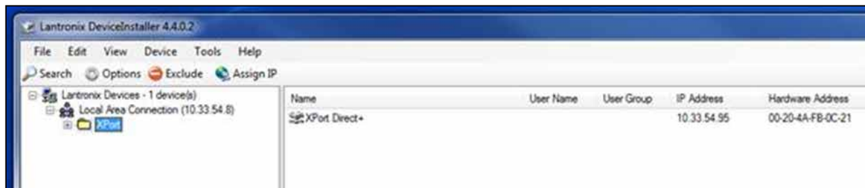
Figure 36 Finding the IP address of a Reader
