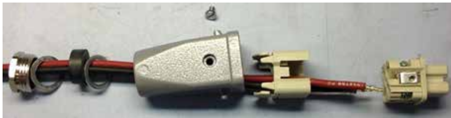
Figure 14 Thread Wires Through Assembly
