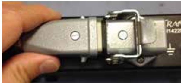
Figure 23 Remove Plug from Receptacle
