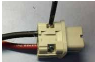
Figure 15 Thread Wires Through Assembly
