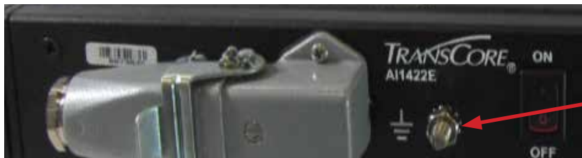
Figure 24 Location of Ground Stud
