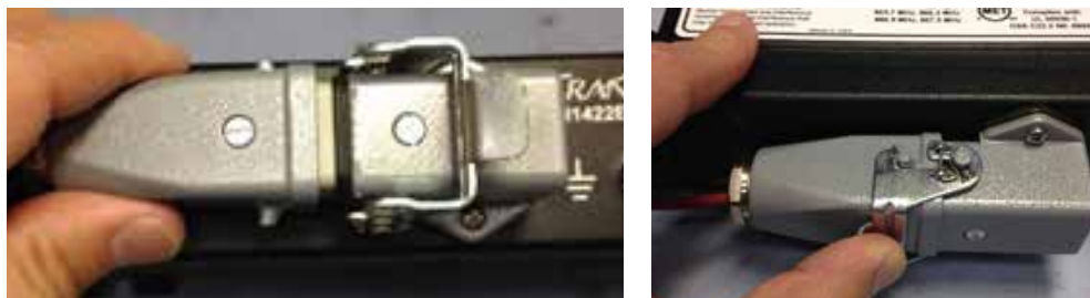
Figure 20 Reinstall Power Connector
