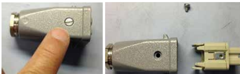
Figure 10 Remove Screw and Plug Insert
