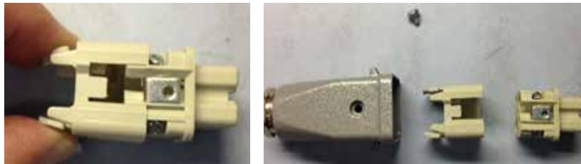
Figure 11 Remove Wire Harness from Insert Clip
