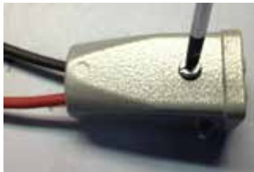
Figure 17 Reassemble and Tighten Set Screw
