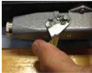
Figure 9 Remove Plug from Receptacle
