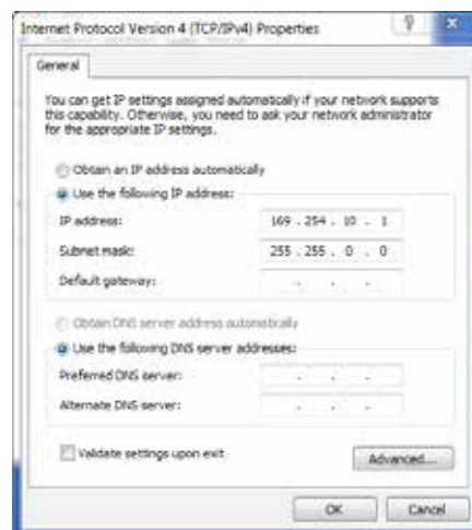
Figure 15 Connecting Directly to Computer Ethernet Port
