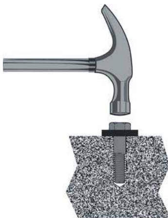
Figure 6 Placing Stud Anchor into Hole
