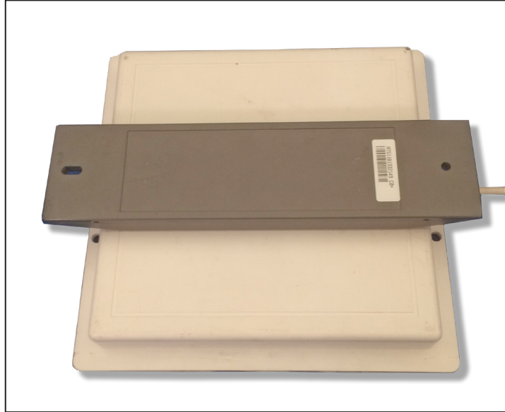
Figure 22 Tag and Antenna Orientation (horizontal polarization)
