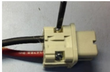
Figure 15 Thread Wires Through Assembly
