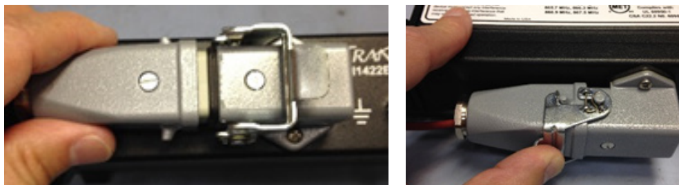
Figure 20 Reinstall Power Connector
