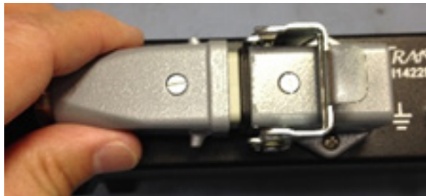
Figure 23 Remove Plug from Receptacle
