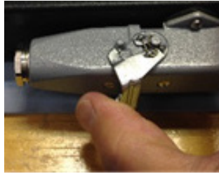
Figure 9 Remove Plug from Receptacle
