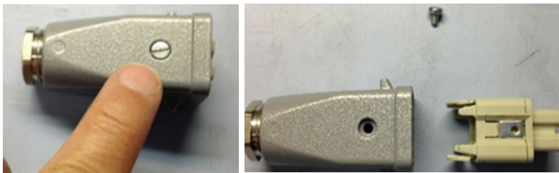
Figure 10 Remove Screw and Plug Insert
