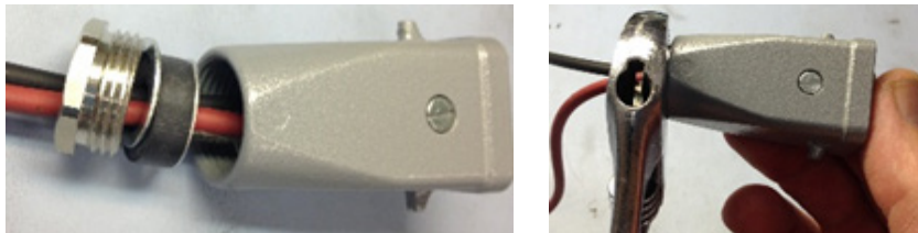
Figure 18 Reassemble Cable Gland Assembly
