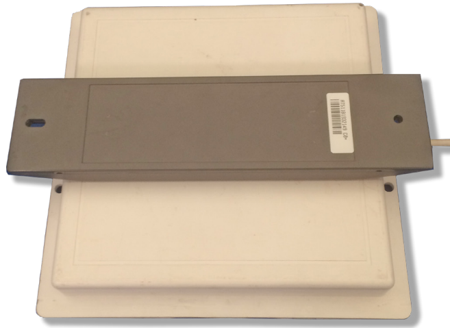
Figure 22 Tag and Antenna Orientation (horizontal polarization)
