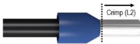
Figure 73 – Proper ferrule crimping position
