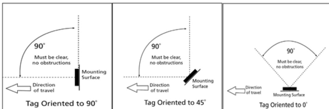
Figure 30 – Guidelines for exterior tag placement
