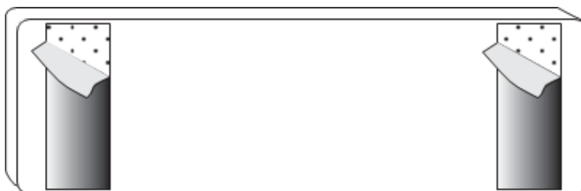
Figure 23 – Remove backing to expose adhesive
