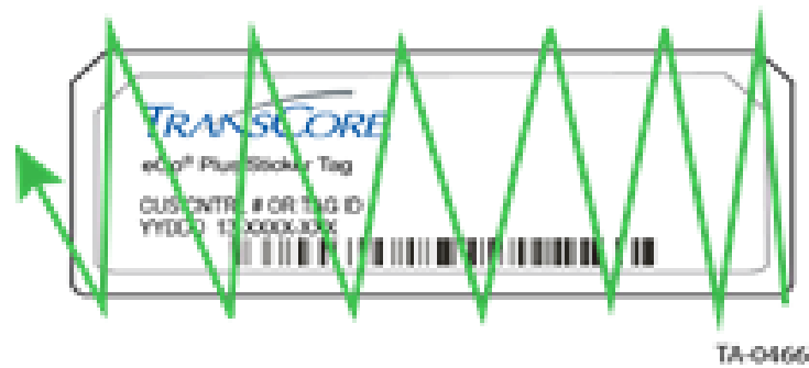
Figure 21 – Rub tag to bond adhesive to windshield
